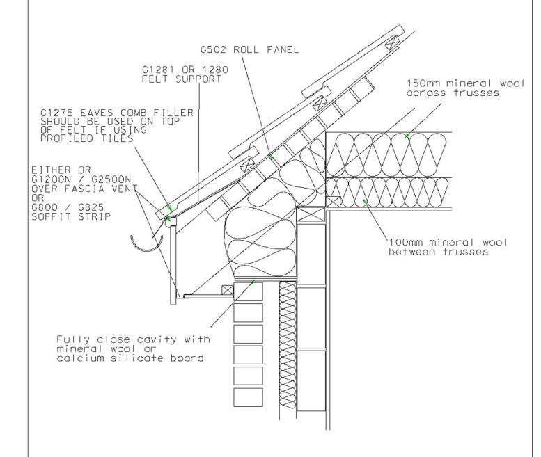
Soffit board ventilation can also be used by removing the Over fascia vent and replacing with G800 or G825 soffit strip clipped to the soffit board depending on 10 or 25mm airflow requirements
