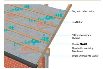
Starting at the edge of the roof and working horizontally, nail or staple BreatherQuilt to the first rafter using 14mm staples, BreatherQuilt should hang down between the rafters ensuring once tile battens are installed a clear 10mm drape is formed at the centre of all rafter spaces.
