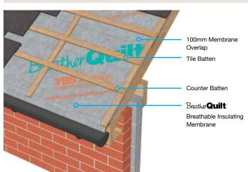
Starting at the edge of the roof and working horizontally, nail or staple BreatherQuilt to the first rafter using 14mm staples, pull taught and proceed across the roof.
