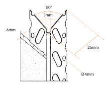
Plaster depth – 6mm Flange width – 25mm Galvanized steel to BSEN 10327-DX51D+Z275
