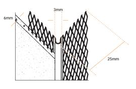
Plaster depth – 6mm Flange width – 25mm Galvanized steel to BSEN 10327-DX51D+Z275
