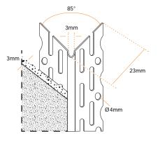
Plaster depth – 3mm Flange width – 23mm Galvanized steel to BSEN 10327-DX51D+Z275
