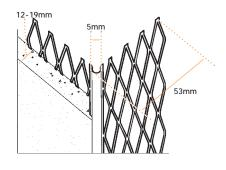
Plaster depth – 12-19mm Flange width - 53mm Galvanized Steel BSEN 10327-DX51D+Z275 Stainless Steel to BSEN 10088-2-1.4301
