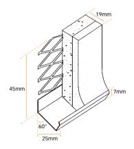
Plaster depth - 16-19mm Flange width – 45mm Galvanized Steel to BSEN 10327-DX51D+Z275 Stainless Steel to BSEN 10088-2-1.4301
