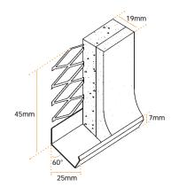
Plaster depth – 16-19mm Flange width – 45mm Galvanized Steel to BSEN 10327-DX51D+Z275 Stainless Steel to BSEN 10088-2-1.4301
