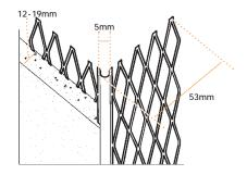
Plaster depth – 12-19mm Flange width – 53mm Galvanized Steel BSEN 10327-DX51D+Z275 Stainless Steel to BSEN 10088-2-1.4301
