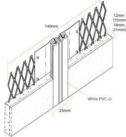
MB 13, 16, 19 dimensions in brackets. Plaster depth – 12mm, 15mm, 18mm, 21mm Flange width - 65mm Galvanized Steel to BSEN 10327-DX51D+Z275 Stainless Steel to BSEN 10088-2-1.4301
