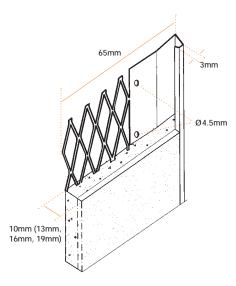
PS 13, 16, 19 dimensions in brackets. Plaster depth - 10mm, 13mm, 16mm, 19mm Flange width - 65mm Galvanized Steel to BSFN 10327-DX51D+7275 Stainless Steel to BSEN 10088-2-1.4301
