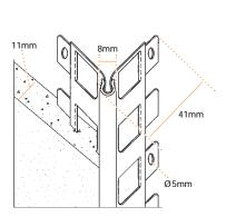
Plaster depth - 11mm Flange width - 41mm Galvanized Steel to BSEN 10327-DX51D+Z275
